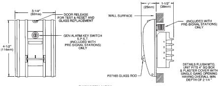
FLUSH INSTALALTION USING P-024900 STEEL BOX
